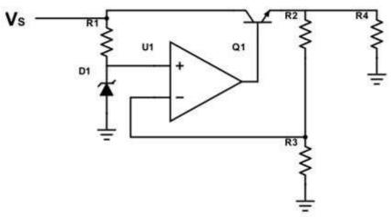
Given that the breakdown voltage is 5V, R1=10k $\Omega$ , R2=100k $\Omega$ , R3=200k $\Omega$ , R4=10 $\Omega$ . The source voltage VS=25V.
