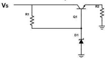
Given that the Zener diode breakdown voltage is 5V, the source voltage is 15V, the output voltage is 10V, R4 =  $2k\Omega$ ,  $\beta$ =99, R1= $2k\Omega$ .
