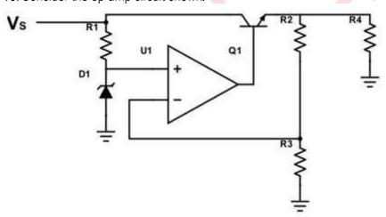
The breakdown voltage of the Zener is 5V.  $\beta$  for the transistor is 100. R1=10k $\Omega$ , R2=90k $\Omega$ , R3=30k $\Omega$ , R4=50k $\Omega$ . Calculate the total output voltage.
